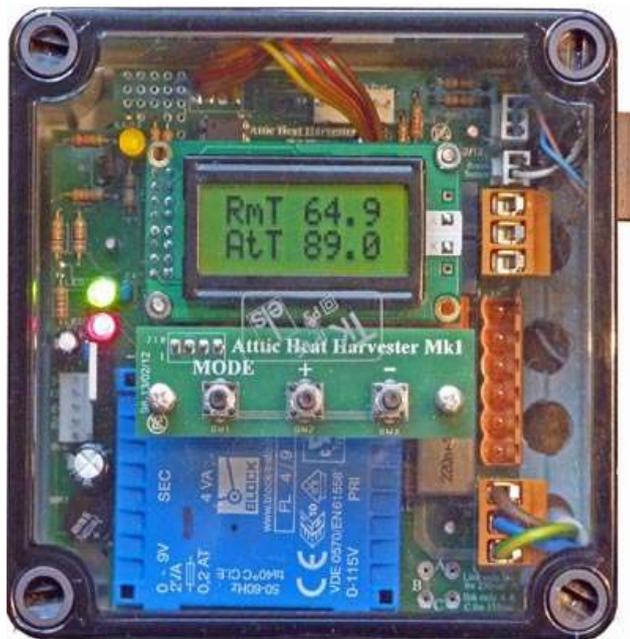
The Attic Heat Harvester Controller has a 2 line back-lit LCD display and 3 key buttons: 'Mode', '+' and '-'.
